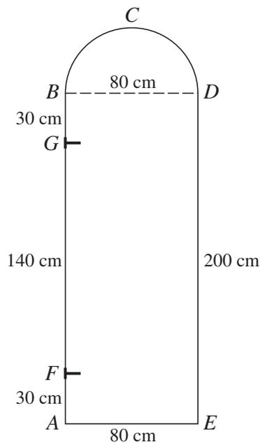
A door is modelled as lamina  $ABCDE$  consisting of a uniform rectangular section  $ABDE$  of weight 60 N and a uniform semicircular section  $BCD$  of weight 10 N and radius 40 cm.  $AB$  is 200 cm and  $AE$  is 80 cm. The door is freely hinged at  $F$  and  $G$ , where  $G$  is 30 cm below  $B$  and  $F$  is 30 cm above  $A$  (see diagram).
