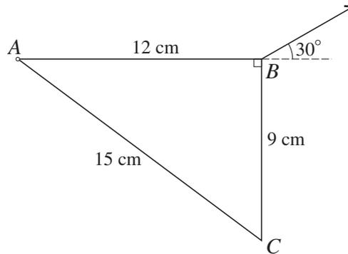
A uniform right-angled triangular lamina  $ABC$  with sides  $AB = 12 \text{ cm}$ ,  $BC = 9 \text{ cm}$  and  $AC = 15 \text{ cm}$  is freely suspended from a hinge at its vertex  $A$ . The lamina has mass 2 kg and is held in equilibrium with  $AB$  horizontal by means of a string attached to  $B$ . The string is at an angle of  $30^\circ$  to the horizontal (see diagram). Calculate the tension in the string. [4]
